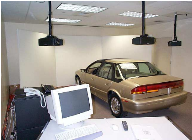
Fig. 3. Components of Driving Environment Simulator: 1995 Saturn, computer for data collection and image generation, three projectors and three screens.
