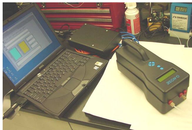
Fig. 6. Portable, field deployable chemical sensing unit.
